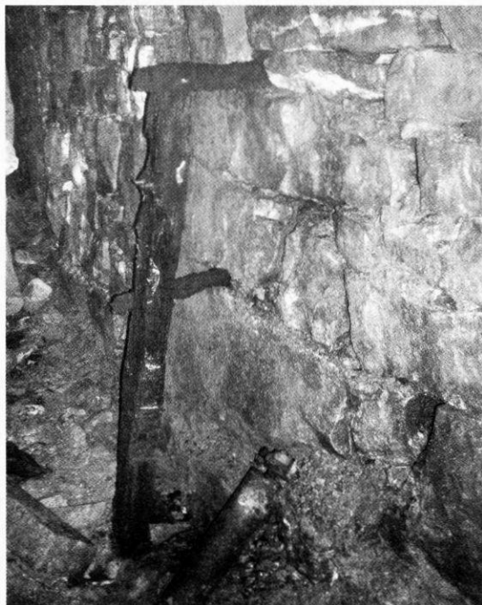
Holmebank Chert Mine, remains of vertical roller in main haulway - Photo by Martin Dixon
